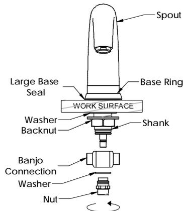
Place backnut onto shank and tighten to underside of work surface.
