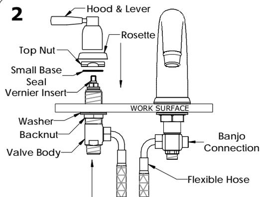
Sidevalve to be installed from underside of work surface as shown.
