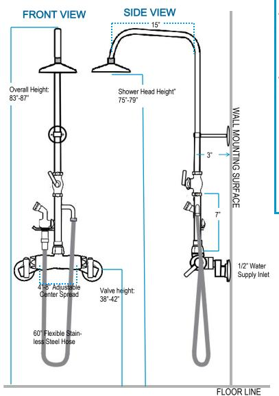
**NOTE:** Flush supply lines before installing valve to remove chips and dirt which can become lodged in the seat washer and cause the faucet to malfunction.
