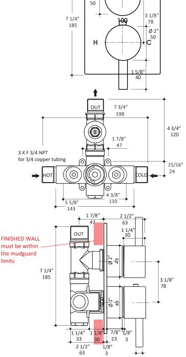
1/2" LACAVA reserves the right to revise any dimension or information on this sheet without notice. Dimensions are nominal and may vary within an industry accepted tolerance of 1/4". Drawings provided herein are meant to give the user an idea of the product and are not made to scale. Location of plumbing is meant for reference, your specific application may vary. 12
