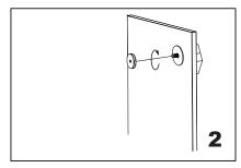
Screw in the fixing bracket into the end cap bolt.
