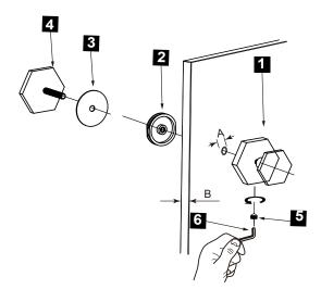
1.Knob x 1 2.Fixing Bracket x 1 3.Clear Gasket x 2 4.End Cap x 1 5.Set Screw M5 x 1 6.Allen Key 2.5mm x 1
