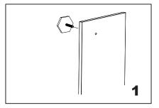
Install the end cap (bolt) through the glass hole, make sure the rubber gaskets are between end cap&glass.
