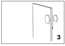
Add the knob on the fixing bracket,make sure the set screw hole in the bottom.
