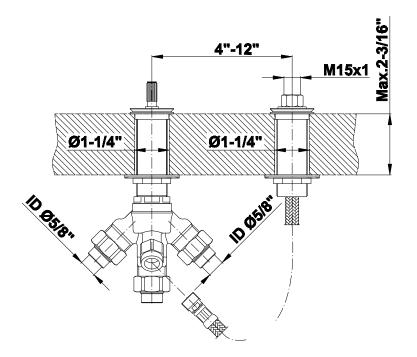
The measurements shown are for reference only. Products and specifications shown are subject to change without notice. Revised 8/2017 <u>www.graff-faucets.com</u> | phone: 800-954-4723 BATHROOM **Qubic Tre Deck-Mounted** Handshower & Diverter Set G-6255-LM39B
