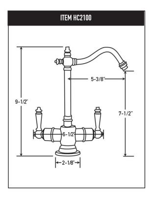
Max Counter Thickness 2" Recommended Installation Hole:
